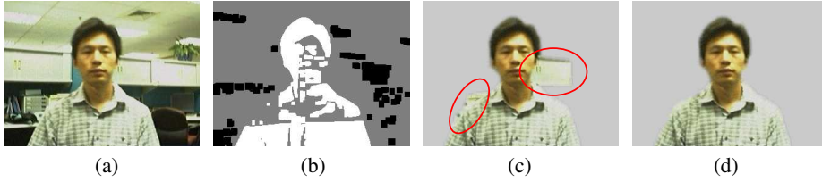
Fig. 2. Foreground layer extraction by different approaches. (a) an image in a video sequence. (b) background subtraction result. Threshold is set to a conservative value to avoid classifying more pixels to foreground. (c) color/contrast-based segmentation result. Red circles indicate notable segmentation errors. (d) our result.
